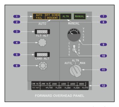
Figure No. 2: Pressurization system control panel
